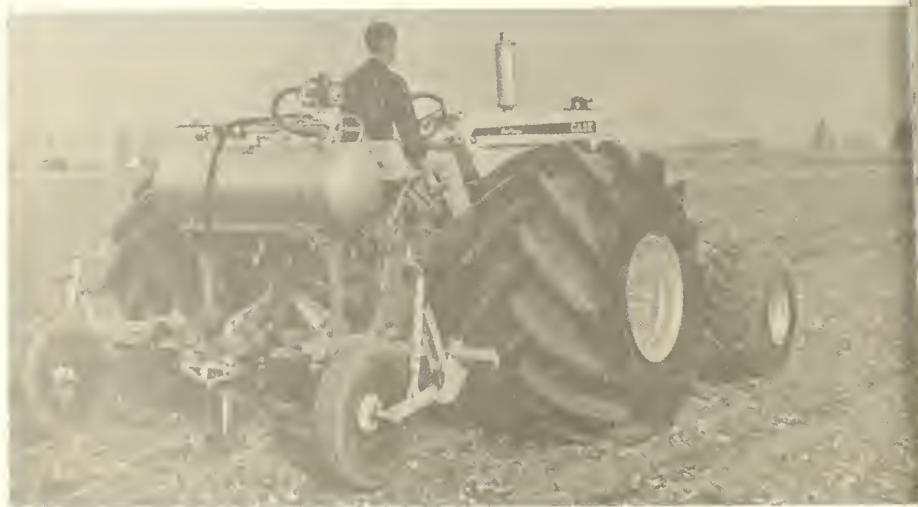
Figure 3. Large floatation-type tires used in early wide-bed studies with a 60-horsepower tractor.
