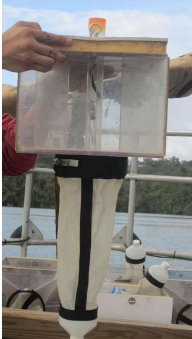
Figure 2.2 Modified quatrefoil light trap.
