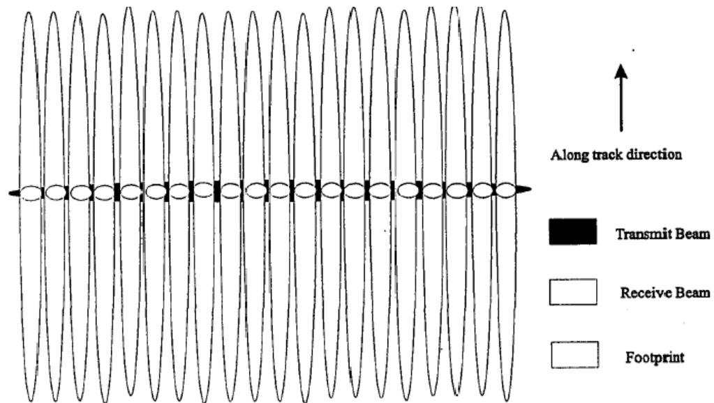
Figure 4.1 Multibeam Transmit/Receive Pattern [1]
