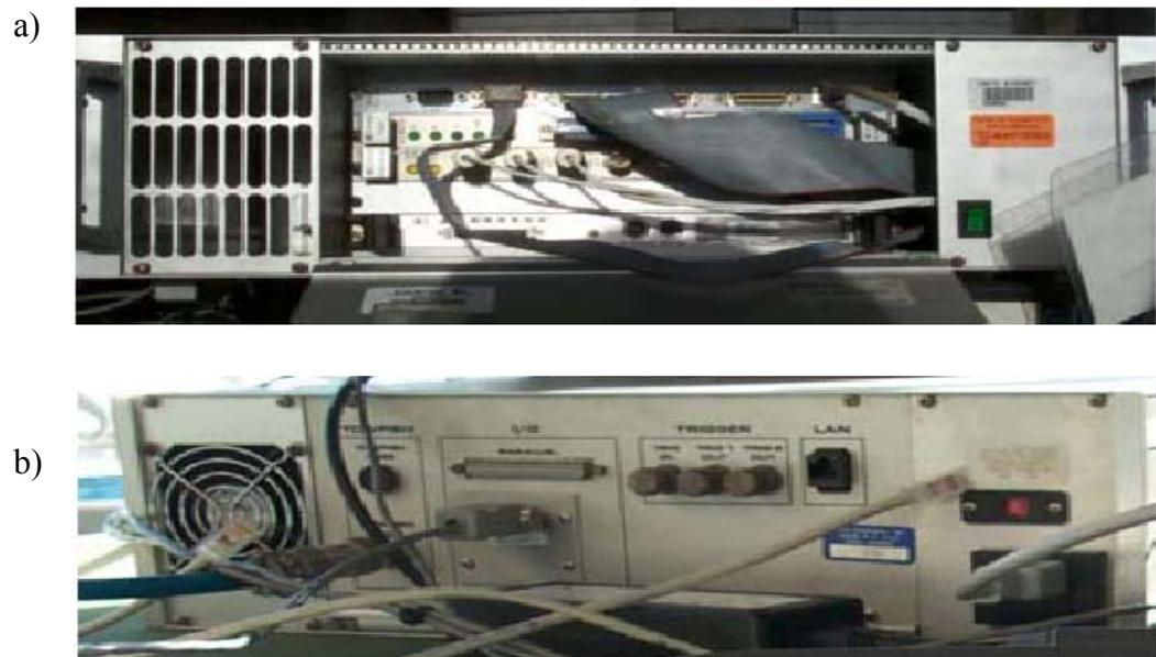
Figure 3.6 The (a) Front View and (b) Back View of the Klein 5500 TPU [5]
