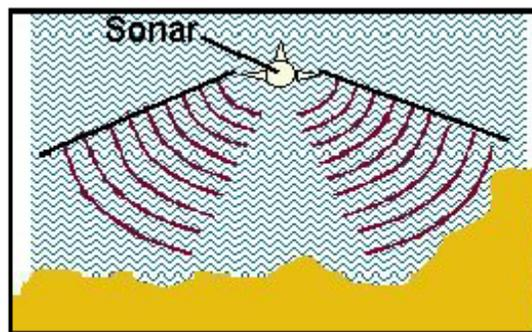
Figure 3.2 Cross-Sectional View of Side Scan Sonar Acoustic Beam showing the Across Track Direction [5]
