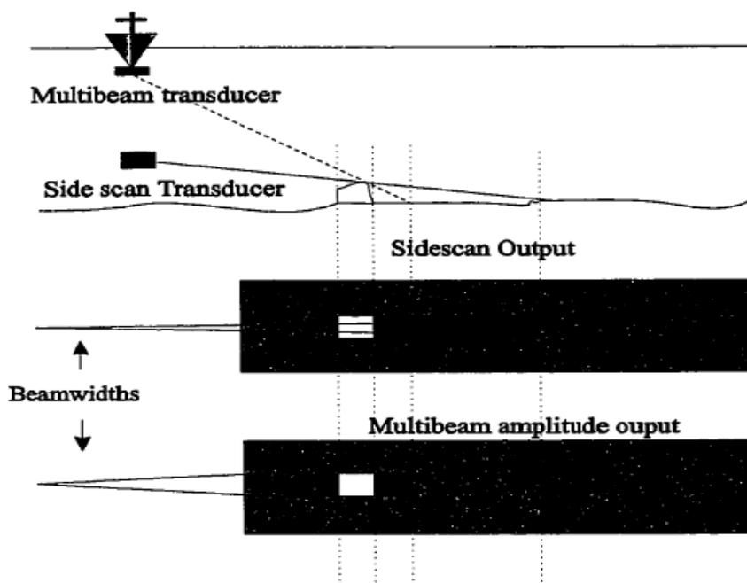
Figure 4.3 Difference in Side Scan and Multibeam Grazing Angles
