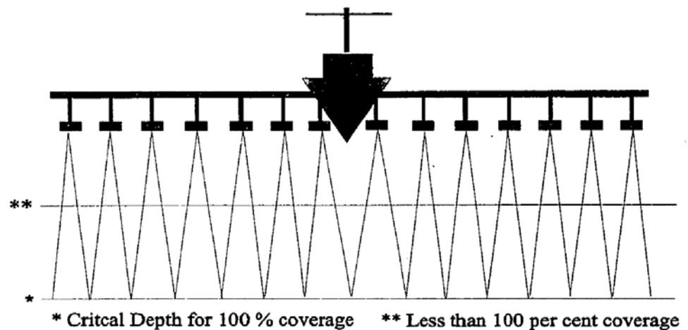
Figure 4.2 Multi-transducer configurations [1]
