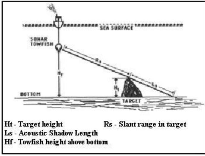
Figure 3.4 A Schematic Diagram of a Sidescan Sonar's Across Track Geometry showing how a Target's Height above the Riverbed is calculated [5]
