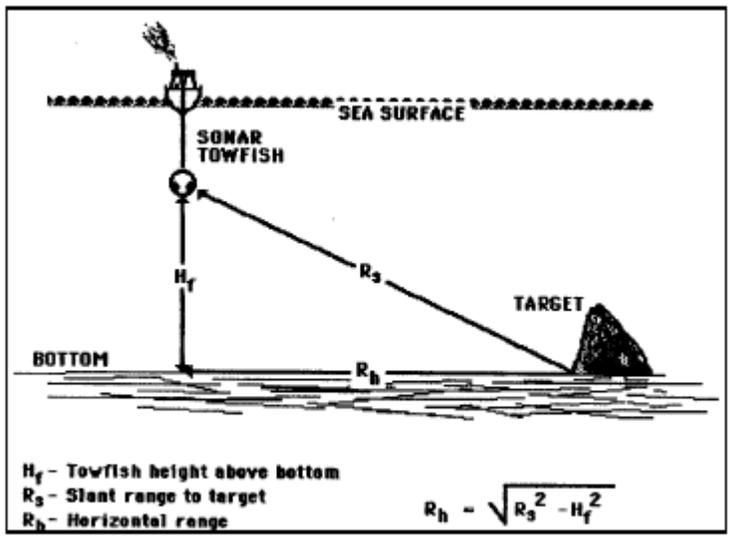
Figure 3.3 Schematic Representation Showing How the Horizontal Distance of a Target from the Nadir of the Sonar is calculated
