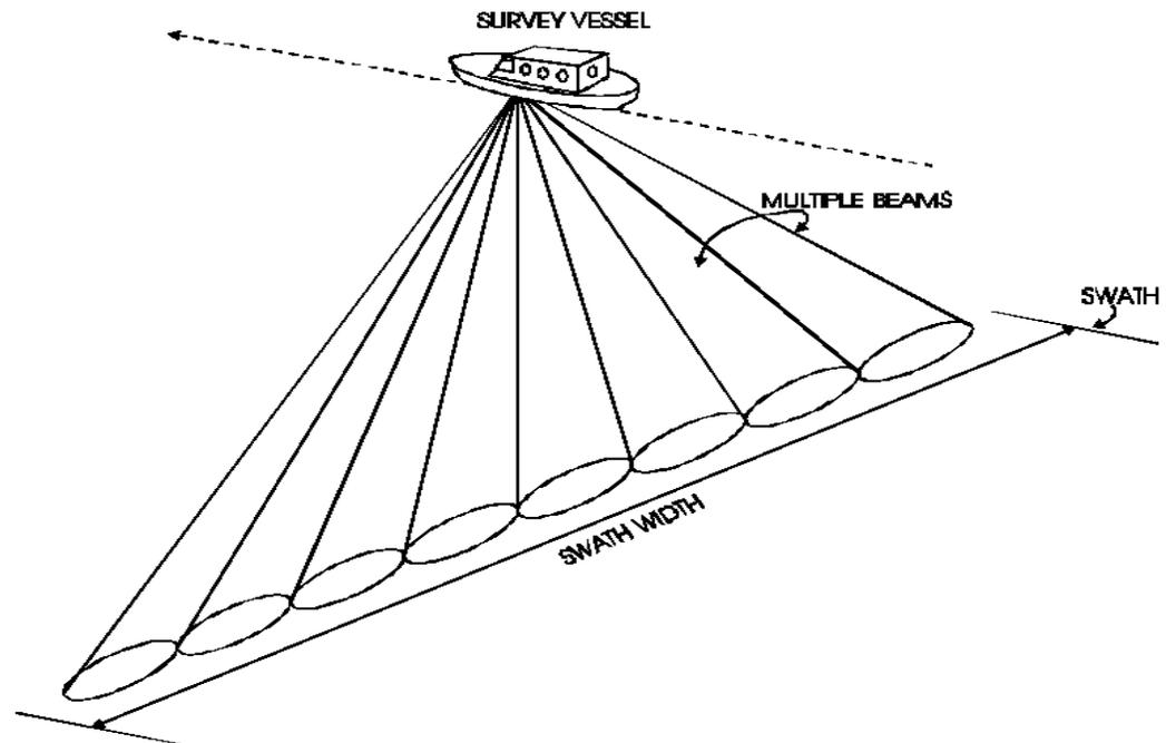
Figure 2.4 Multibeam Sonar Showing Swath
