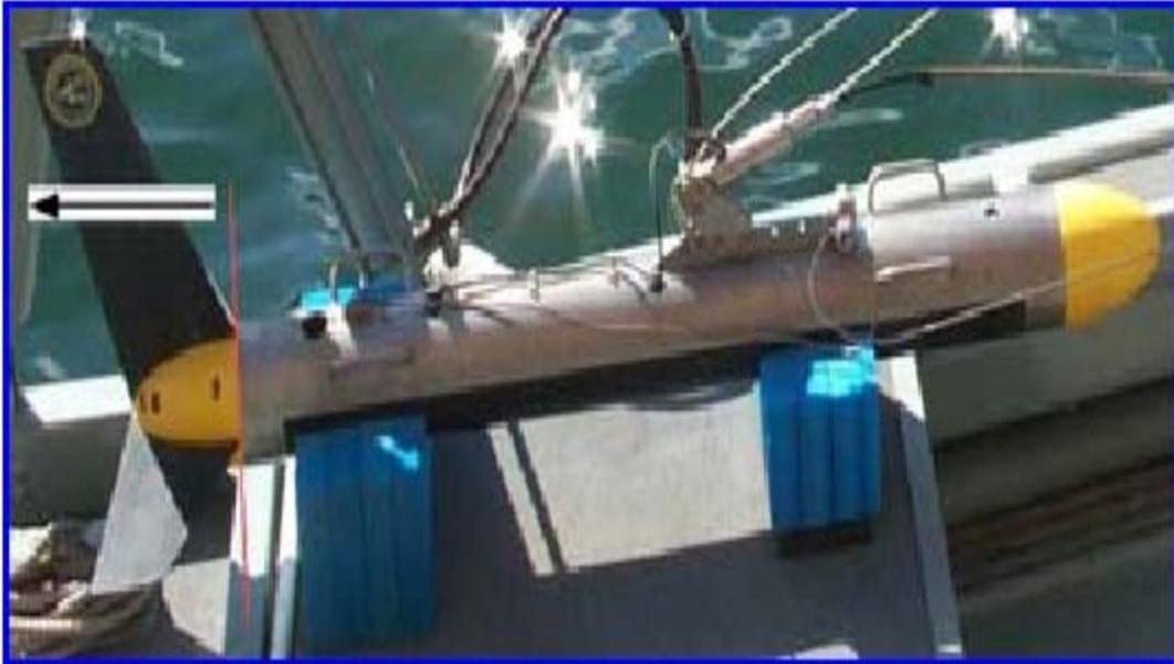
Figure 3.5 The Klein 5500 Sidescan Sonar Showing Where The Rear Yellow Nose Cone, Housing the Tail Fins, will Separate (Indicated by Red line) From the Stainless Steel Body When the Tail Fins become Snagged on Any Bottom Objects [5]
