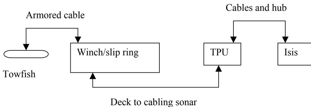
Figure 3.7 Flow Diagram Showing the Hardware Setup for the Klein 5500 sidescan sonar
