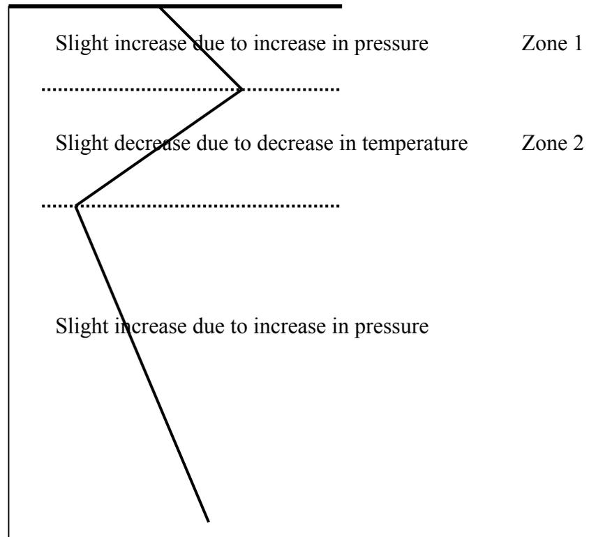
Figure 2.5 Vertical Profiles of Temperature and Sound Velocity
