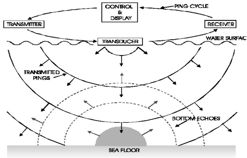
Figure 2.3 Components of Single Beam Depth Sounder System
