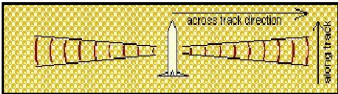
Figure 3.1 Plan View of the Acoustic Beam Generated by a Sidescan Sonar Showing its Narrow Along Track Characteristic [5]
