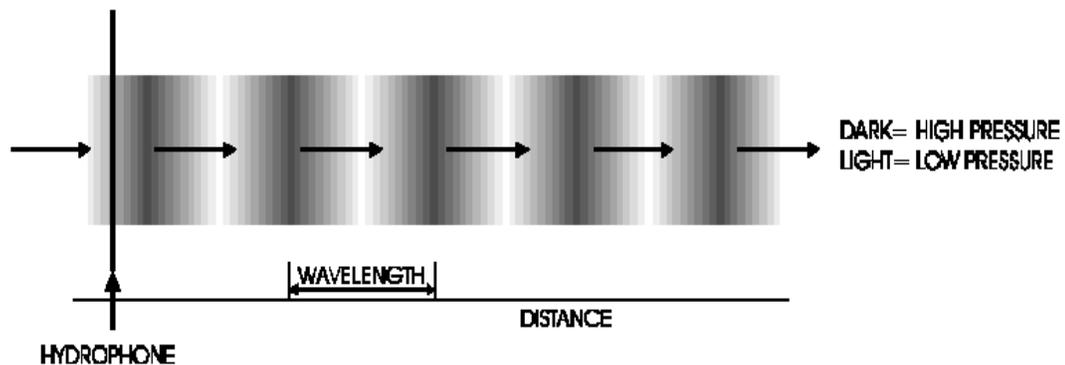
Figure 2.1 Components of Sound Wave [8]
