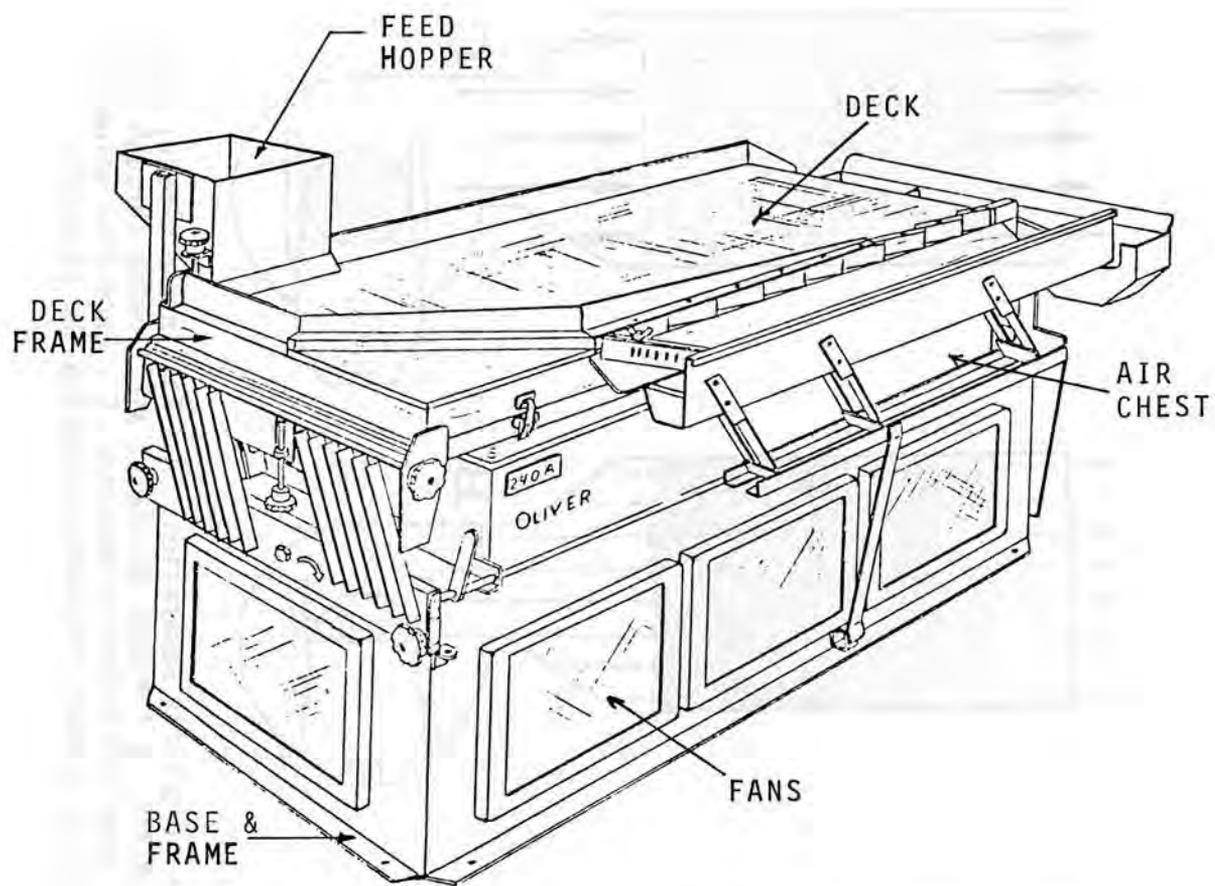
Figure 1. Diagram of a gravity table.
