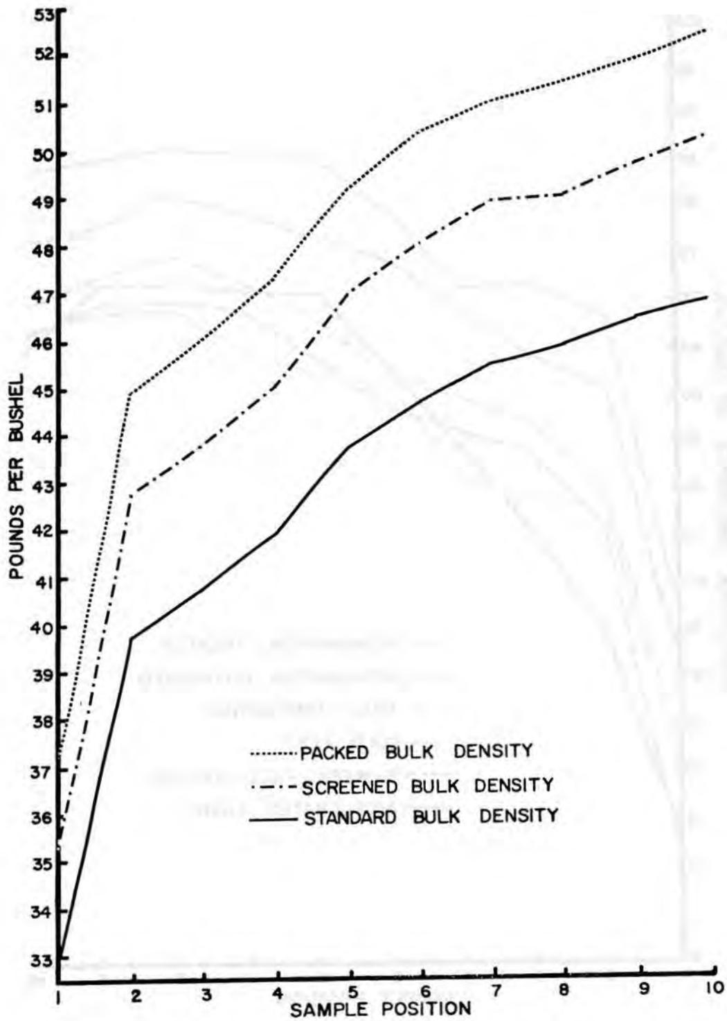
Figure 4. Average density (pounds-per-bushel) of cottonseed over 10 positions across the discharge end of a gravity separator. (Gregg, 1969).
