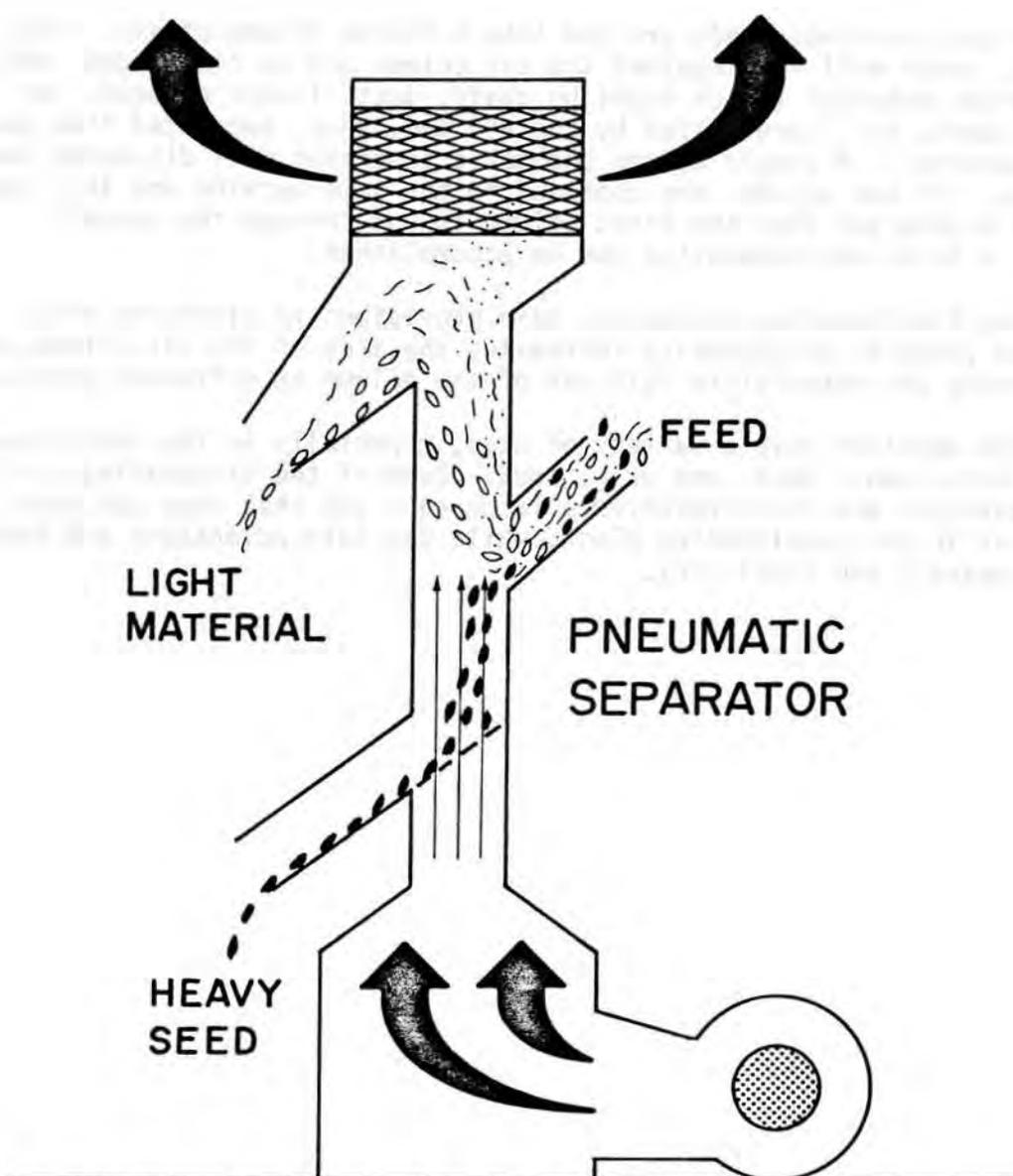
Figure 8. Flow diagram of a pneumatic separator.
