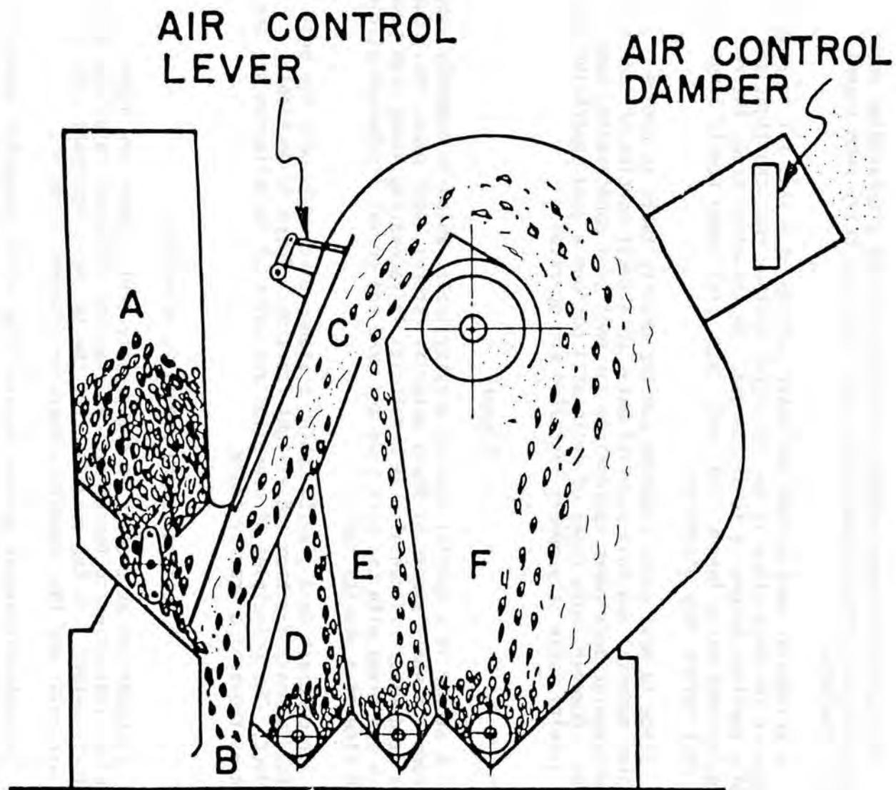
Figure 7. Flow diagram of a fractionating aspirator.
