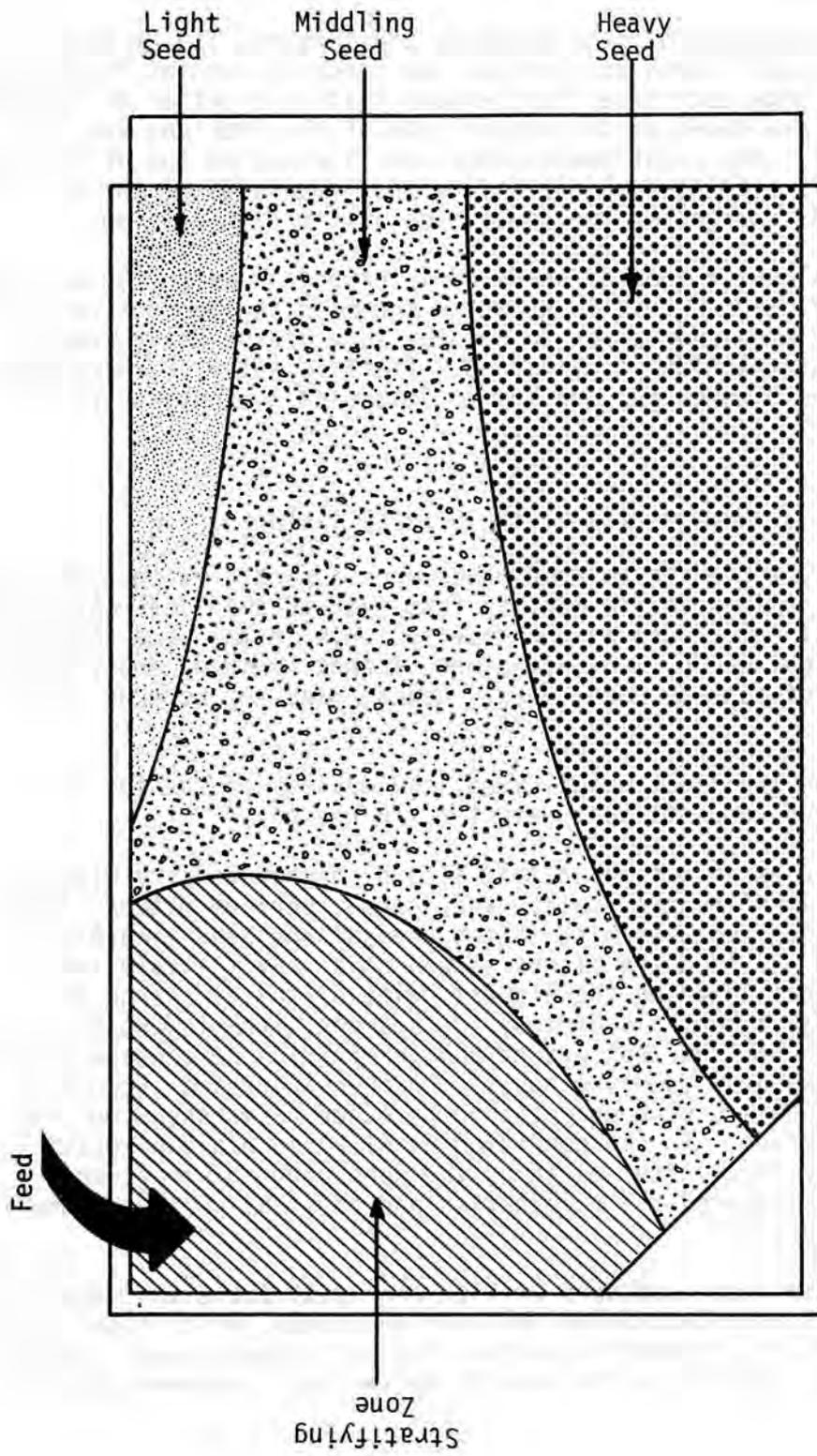
Figure 3. Top view of gravity table showing flow pattern of seed across the deck.
