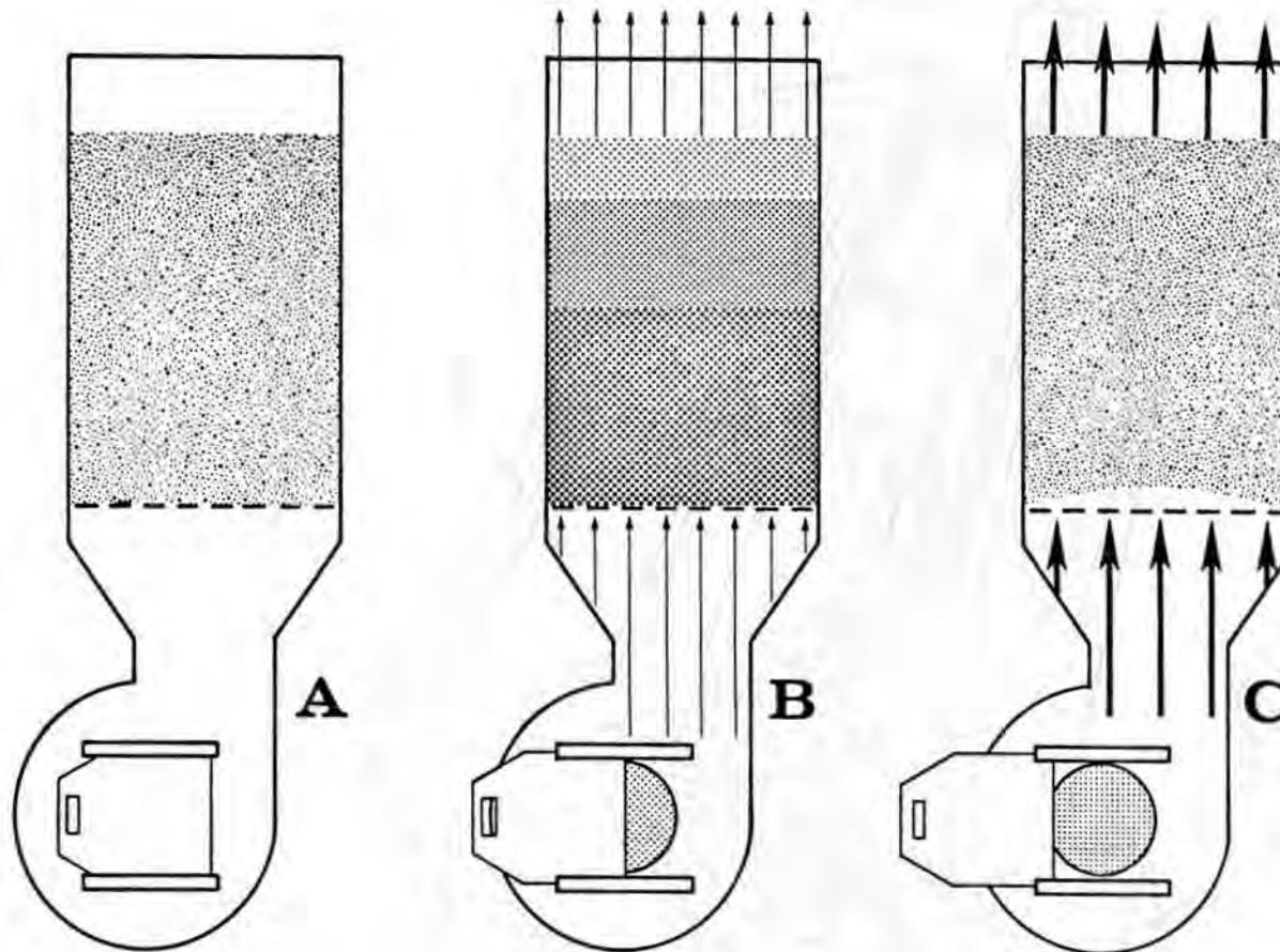
Figure 2. Principles of gravity separation. A - Fan intake closed; no stratification. B - Proper volume of air flowing through the deck; seed stratified by density. C - Excessive volume of air flowing through the deck disrupting the stratification.
